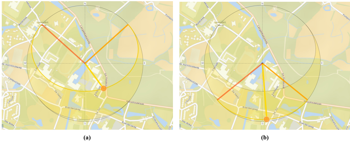
Figure 4.2: Sun trajectories in (a) summer solstice on the 21st of June (b) winter solstice on 21st of December.
