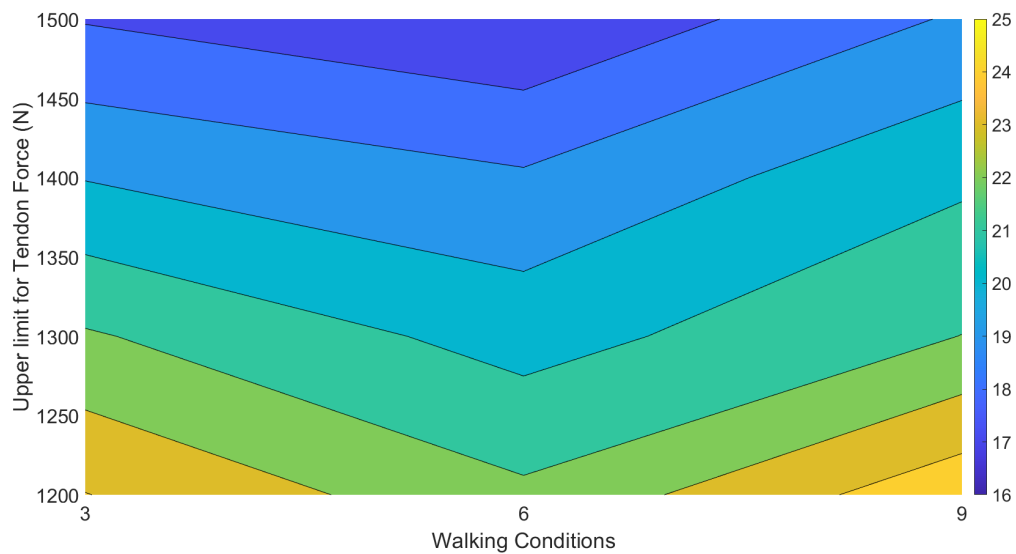
Figure 5.17: This contour plot indicates the reduction percentage in peak tendon force for a variety of walking conditions (Elevation = 20%)
