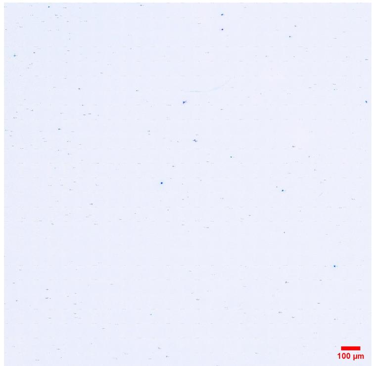
(d) The stitched picture of all microscope pictures of the first experiment of area 1. After Python analysis and inverted.
