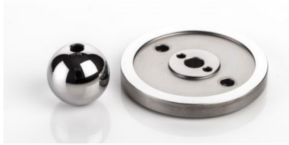
Figure 21: Specimens for the MTM machine. Left the ball and on the right the disk, obtained from [59].
