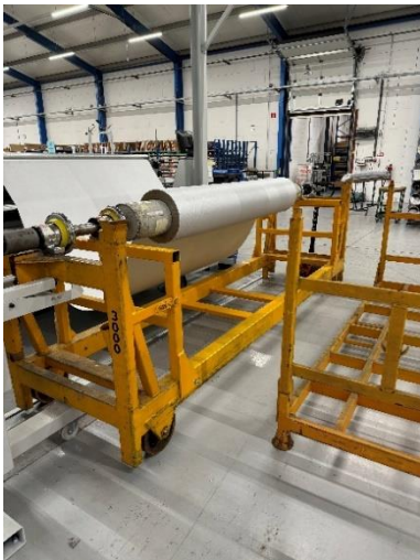
Figure 29: Jumbo Roll Structure Holding It
