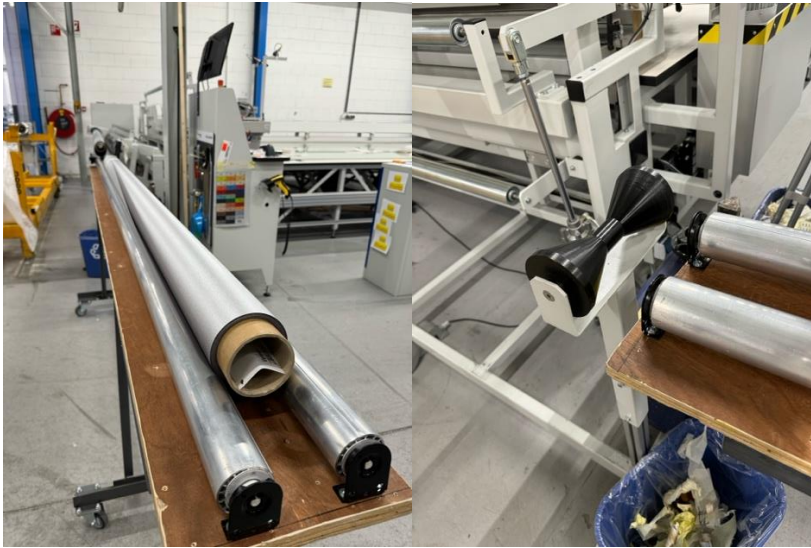
Figure 26: Hand-made Fabric Holding Table (Left). Close-up Table to Fabric Feeder (Right)
