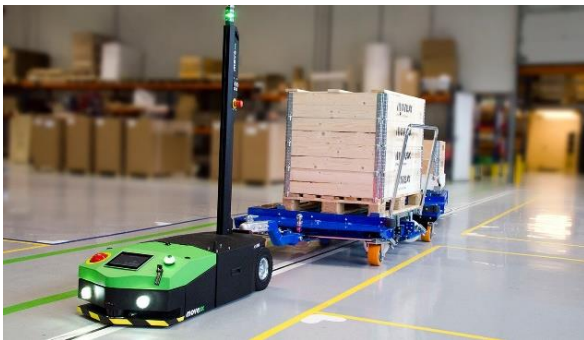
Figure 24: Automated Cart System. Adapted from https://movexx.com/nl/9-manieren-waarop-automatisch-geleide-voertuigen-het-goederentransport-efficient-maken/
