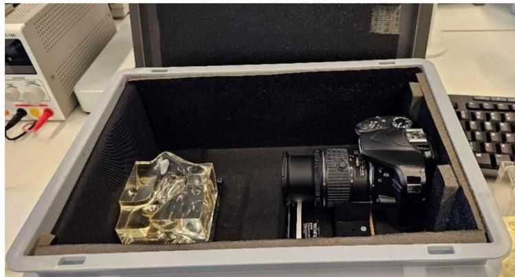
Figure 9: Setup inside the dark box for acquiring images of calcein deposition.
