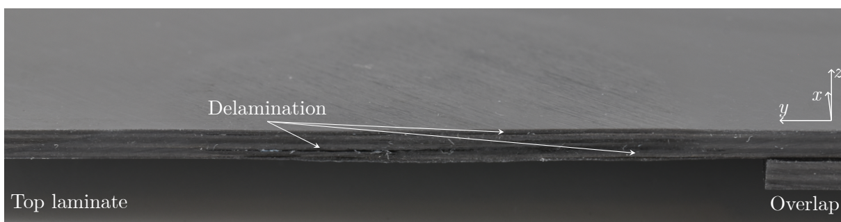
(b) Close-up of an edge effect outside the start, imaged from the top.
