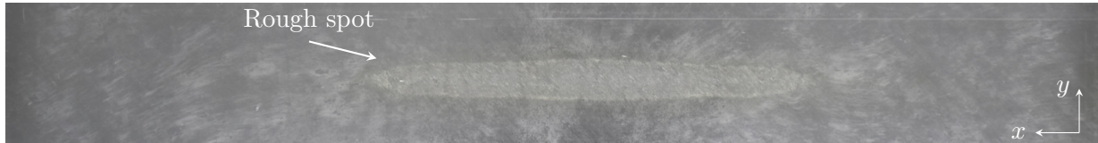
(a) Bottom surface of the reference assembly weld overlap (B1L1) showing a rough spot.
