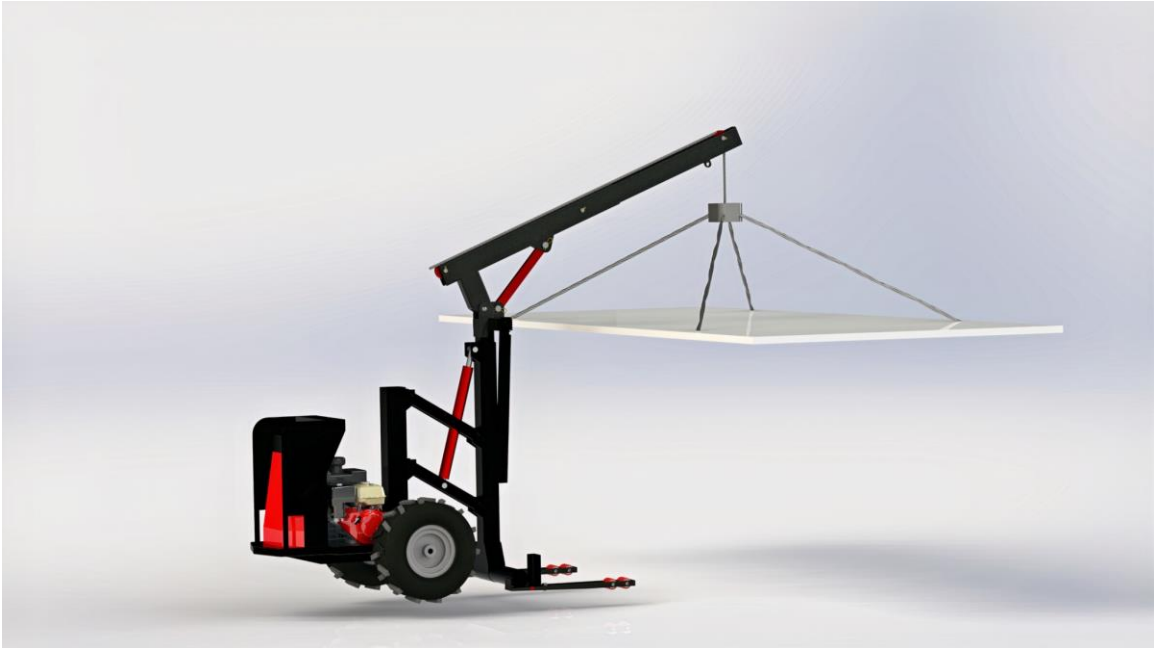
Figure 5 - Redesigned Cardinal mule lifting the roof
