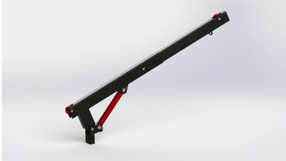
Figure 3 - Final design crane boom with connection part
