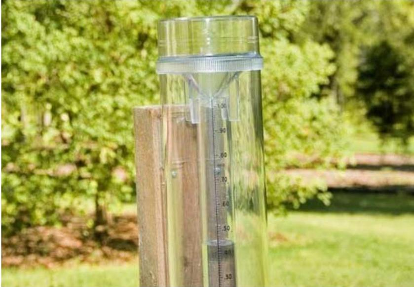
**climate.news** Rain gauges are the most common instrument used to measure rainfall. A rain gauge is an open-at-the-top container that is calibrated to measure the depth of liquid caught. In the United States, the depth of precipitation is reported in inches. Satellite instruments can also detect and estimate precipitation amounts. #RainfallMeasuring #Climate
