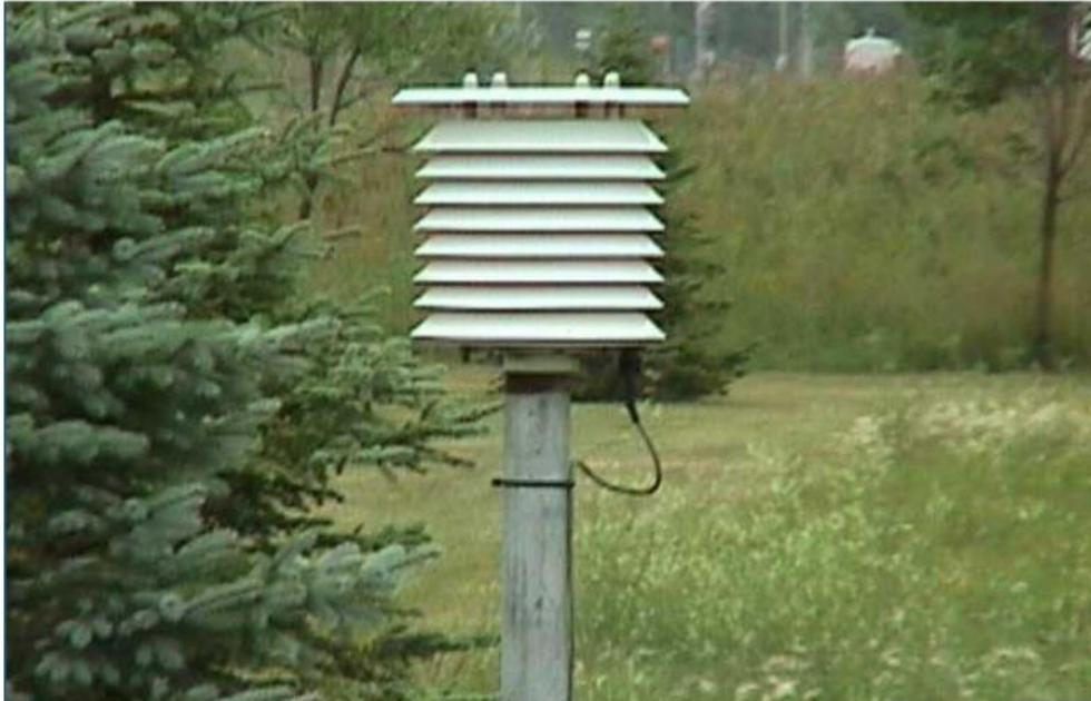
**climate.news** Climate is measured by observing air, land, and ocean. Surface air temperature, typically taken about 2 meters above the ground, is measured with thermometers shielded from sunlight. The common type is the liquid-in-glass thermometer, while more precise ones, like the air temperature sensor shown on the photo, check electricity through metal samples. #Climate #ObservingAir #ClimateAndWeatherMeasurement
