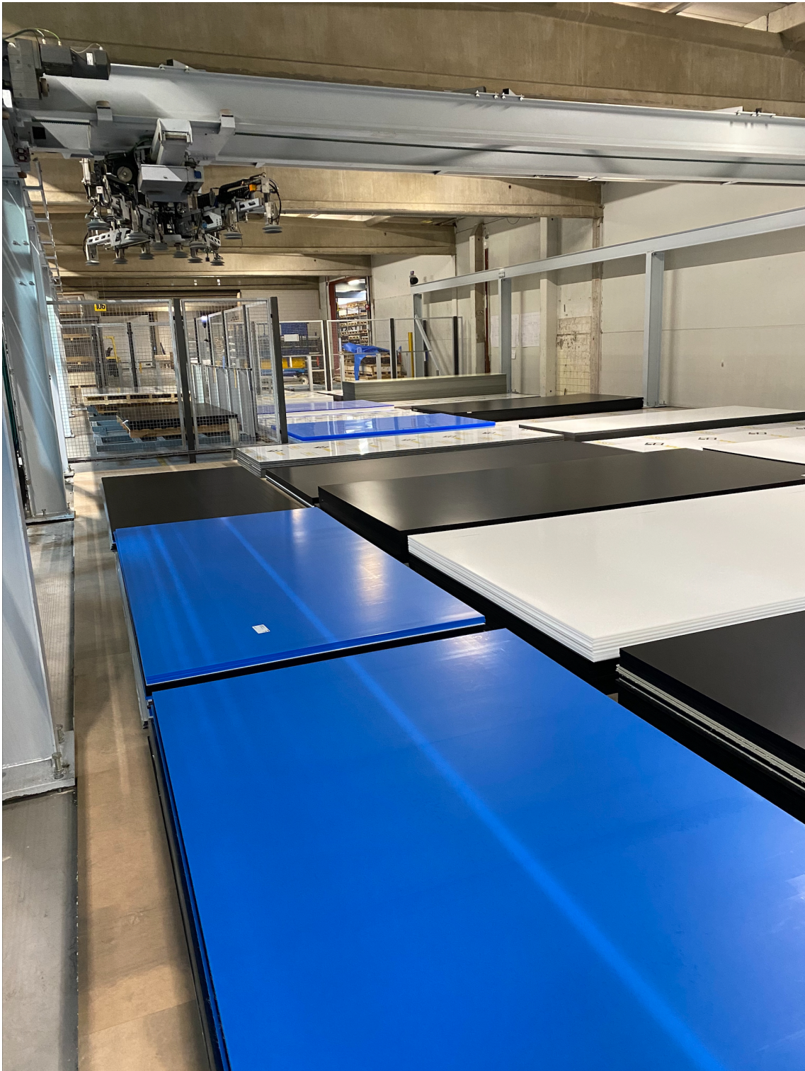
FIGURE A2: System with crane and stacks
