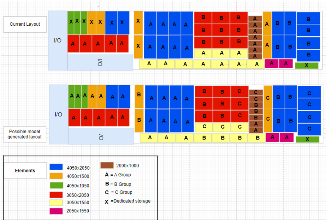
FIGURE 2.8: Current AS/RS layout and possible layout generated by the model for reducing total travel time.
