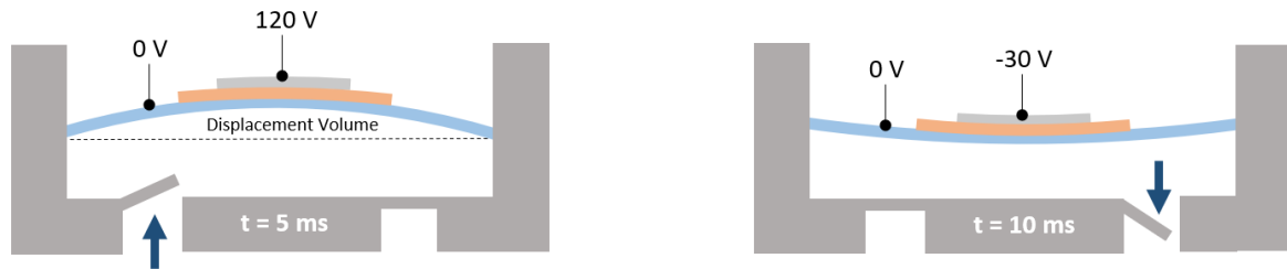
Figure 4.2: Utilization of the Piezoelectric Effect within Micro-Pump at a Frequency of 100 Hz.
