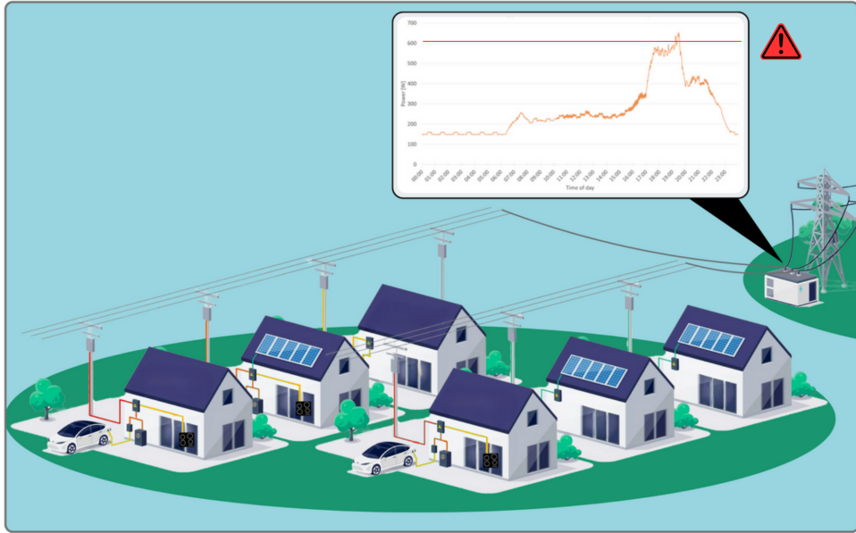
FIGURE 5.1: Example of cable and transformer overloading in a visualization.
