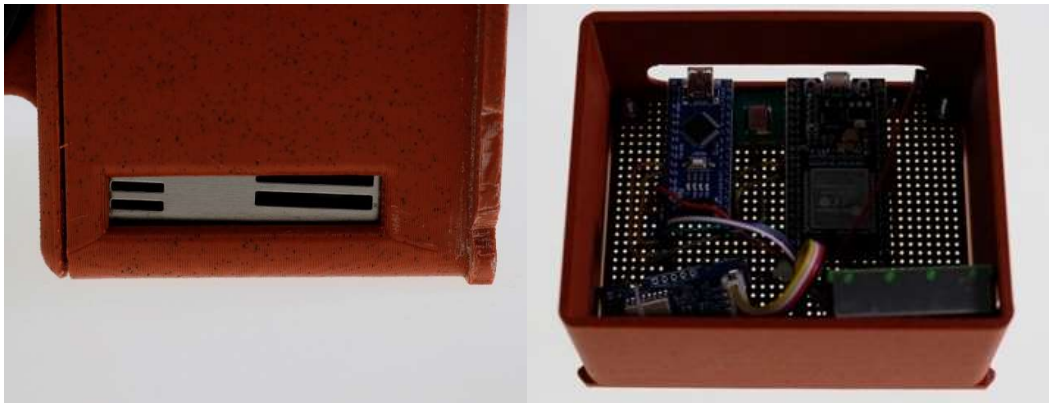
Figure 15: Openings on the casing for the air pollution airflow (left) and USB access (right)
