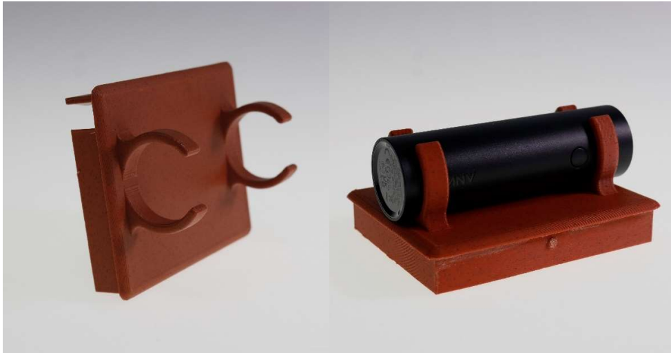
Figure 16: Casing cover for the external battery holder
