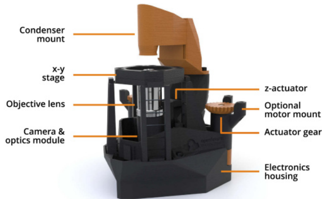
Figure 8: Labelled CAD model of the OpenFlexure design by Collins et al.[11].
