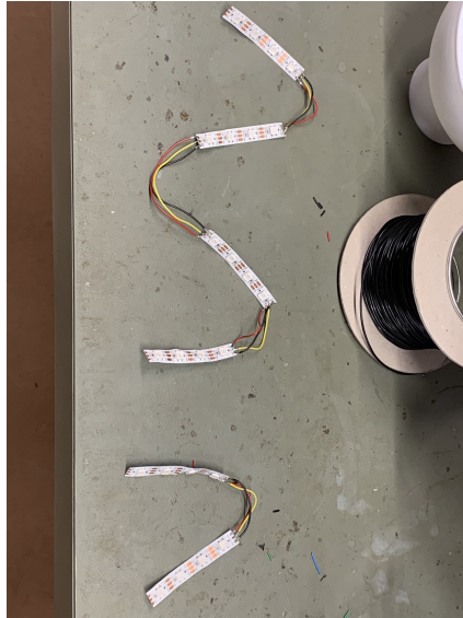
Figure 22: LED strips in the process of being connected using soldering.
