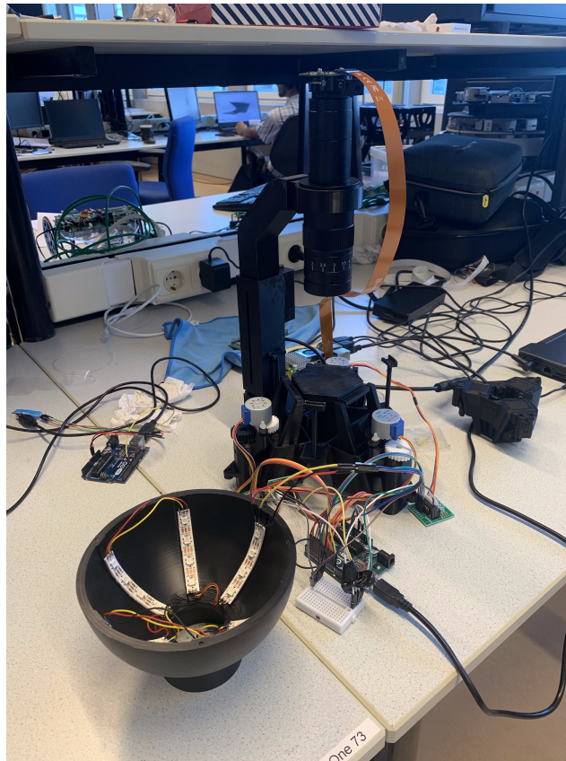
Figure 24: Realisation of the microscope hardware in non-RTI configuration. The RTI dome is shown in front.
