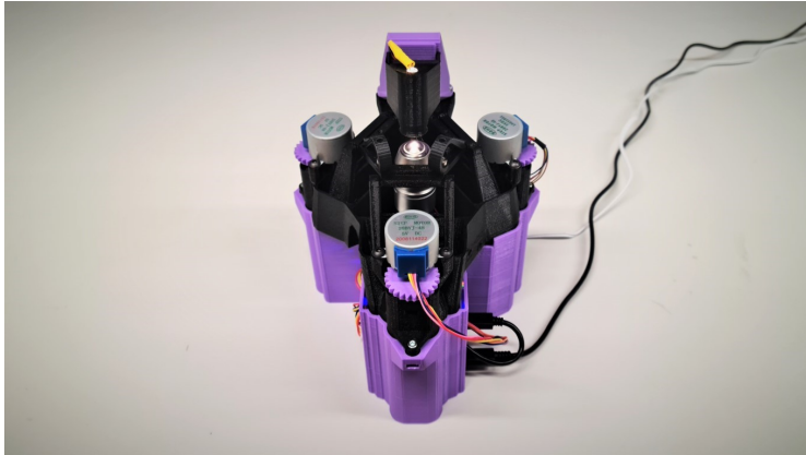
Figure 17: A 3D-printed OpenFlexure Delta stage, image from McDermott et al.[12].
