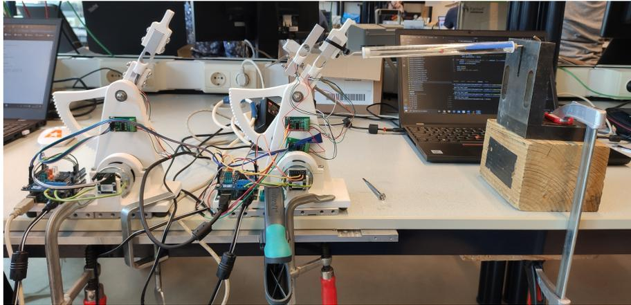
**Figure 5.7:** Measurement setup used in experiments 5.2, 5.3 and 5.5 to measure the transparency in terms of position and force tracking when interacting with (one end of) a spring.
