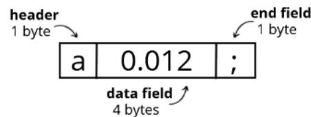
**Figure 3.4:** Overview of the messages' fields (and their sizes) that are communicated in "string" format between the Arduino and Processing interface [50].
