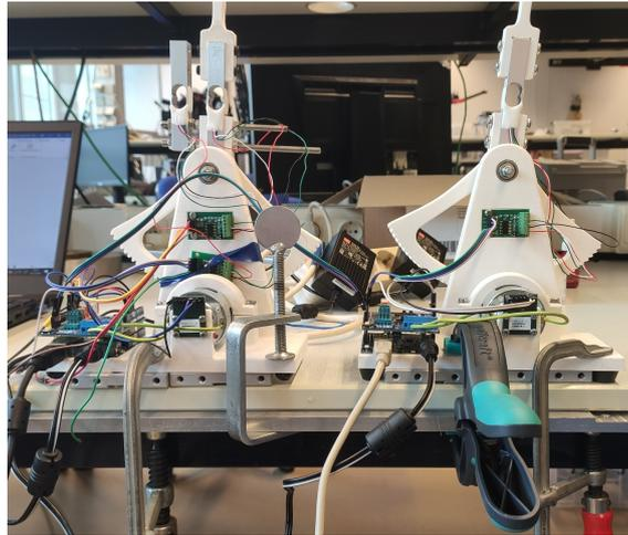
**Figure 4.16:** Measurement setup used in experiment 4.4 to determine the optimal proportional gains ( $K_p$ ) for the position-measured force and position-computed force architectures.
