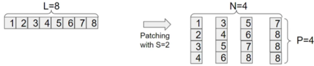
Fig. 4. By setting patch length( P ) = 4 and stride( S ) = 2 with sequence length( L ) = 8, four patches are generated as shown in this figure.
