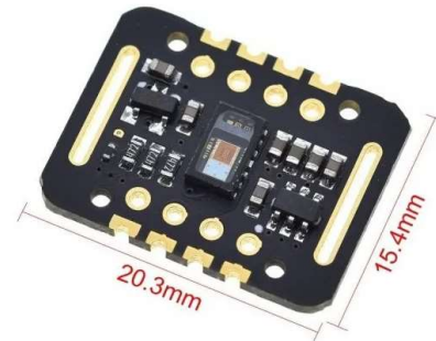
Figure 15, The MAX30102 (OT3546) pulse oximetry board [7].
