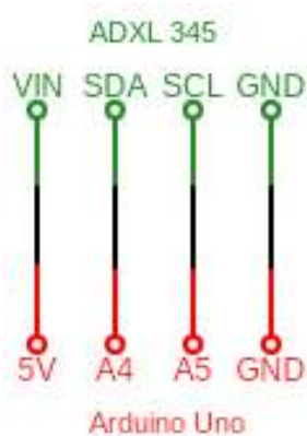
Figure 39, Circuit of test setup for the ADXL345 sensor.
