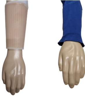
Fig. 2. TSP-equipped mannequin arm without (left) and with a sleeve (right)
