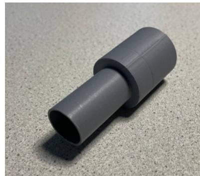
Figure 30 3D printed part for attaching the slip ring to the pole
