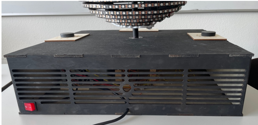
Figure 28 Back panel of the installation
