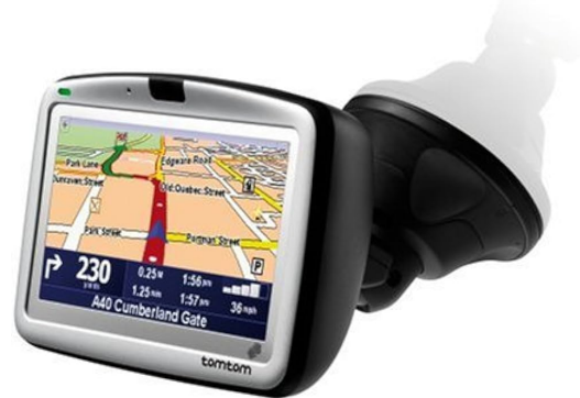
Fig. 1. Tom Tom 910, one of the first in-car Navigation Systems to feature text-to-speech synthesis technology [4]
