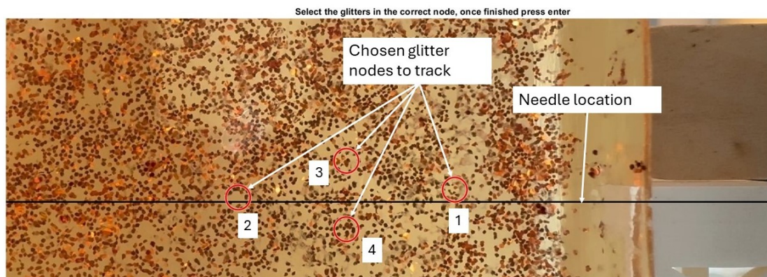
Figure 5.15: The 4 locations in the phantom where glitters are traced over time to find the deformation.
