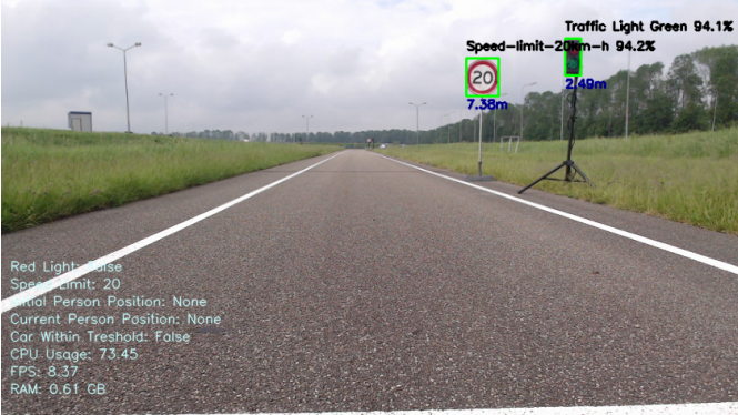
Fig. 8: A visualisation of what the model detects, the detections boxes are drawn as green rectangles around objects, where around it has the class that it detects and the distance calculated towards it
