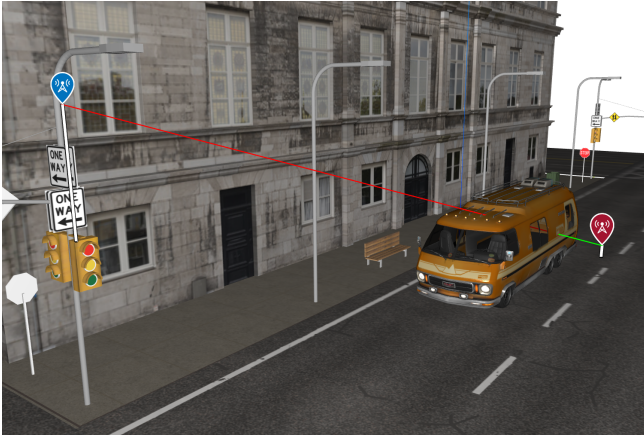
Fig. 2. Line-of-Sight path between the tx and rx antennas
