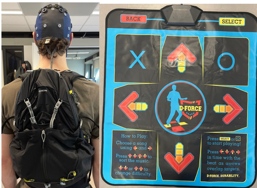
Figure 3. Mobile EEG system and D-Force dance mat. EEG was recorded from channels FPz, FCz, F9, F3, F4, F10, Cz, M1, T7, C3, C4, T8, M2, P9, P7, P3 Pz, P4, P8, P10, Q1, Q2.
