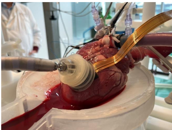
Figure 18: Side view from the right of the PhysioHeart™ platform and structure holding the electrode grid in place.
