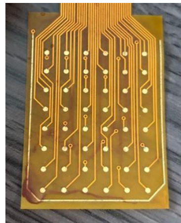
Figure 21: Electrode grid with inter-electrode spacing of 4 mm.
