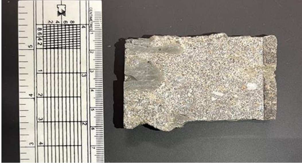
Figure 4. Quartz arenite sandstone core sample used for this study.
