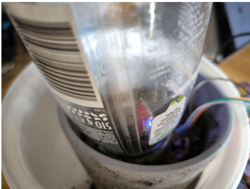
Figure 7.7: CO 2 sensor test enclosed in a glass jar on top of soil.
