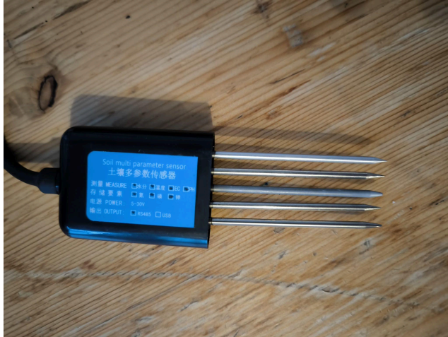
Figure 5.1: picture of the combination sensor used in the prototype.
