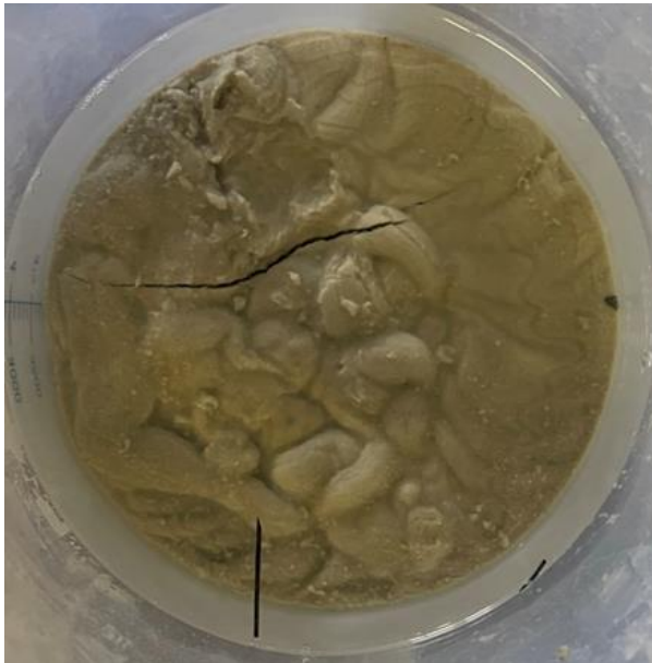
Figure 29, Small-scale experiment saline and lowered pH - Tap water on day 5
