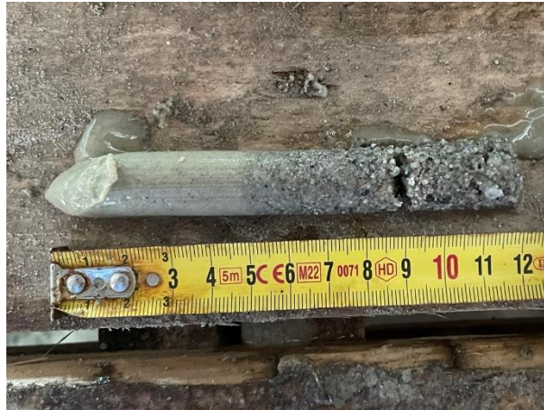
Figure 46, Large scale lowered pH - Sample layer build-up
