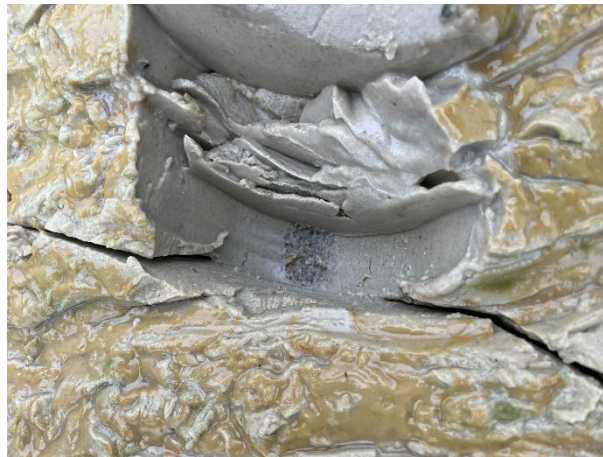
Figure 54, Large scale CaCl 2 - Formation cracks all the way through
