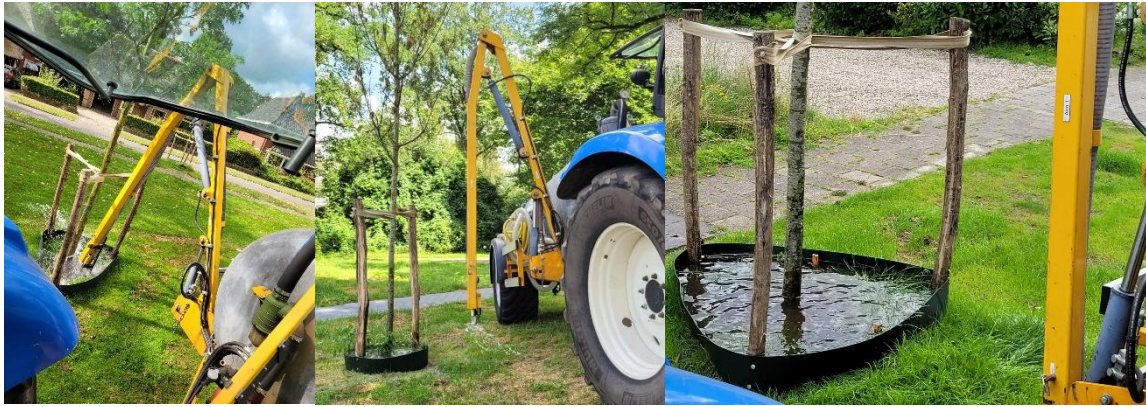
Figure 41, the process of watering a tree at which some visible spilling occurs
