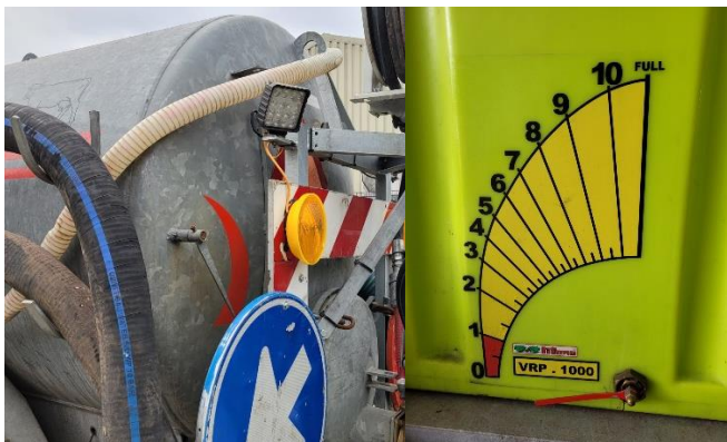
Figure 13. float level gauges present on the equipment of Onderhoud Enschede BV
