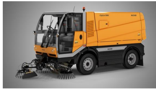
Figure 7, Bucher CityCat 5006 used for street cleaning
