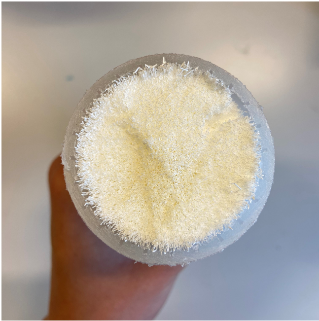
Figure 6: Cross-section image of the FX1000 dialyzer.
