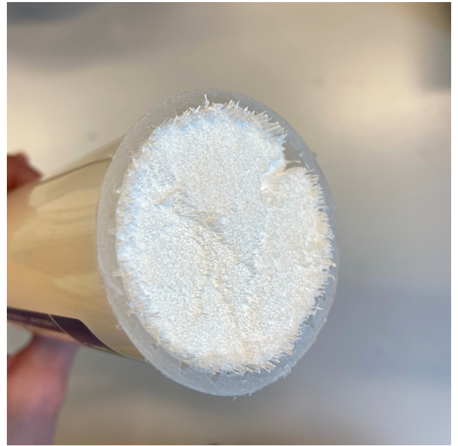
Figure 7: Cross-section image of the FX1000 dialyzer, with a better view of the dialyzer fibers.
