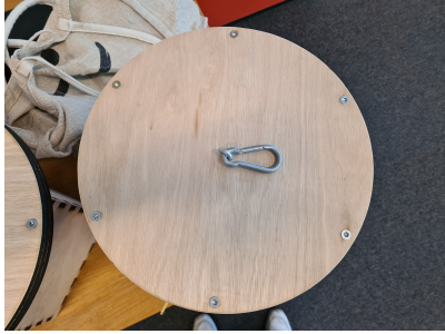
FIGURE 6.2: The top of the prototype with 6 countersunk bolts and a hook to hang it up in the enclosures.
