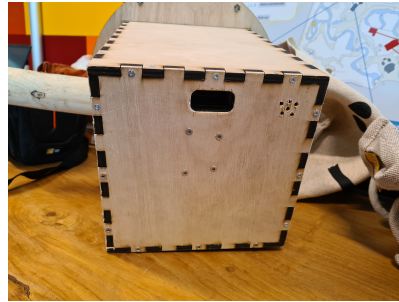
FIGURE 6.5: The bottom of the unit with the feeder hole and some speaker holes.
