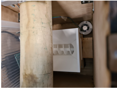
FIGURE 6.4: The feeder system and speaker on the bottom of unit two, same principle for unit one.
