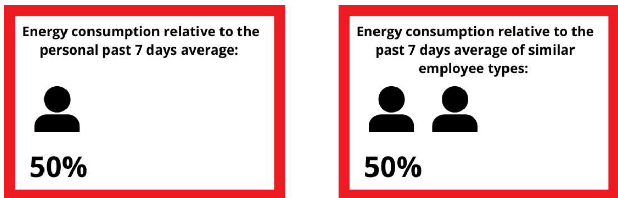
Figure 72: Examples of the buzz pop ups on the screen that is displayed alongside the vibrational feedback.
