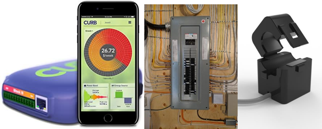
Figure 4: An illustration of curb can be seen in the left picture. The blue box is the hub and transmitter. On the phone the processed data is visualized. In the middle an electrical panel can be found. On the right an example of what a CT clamp looks like is shown.
