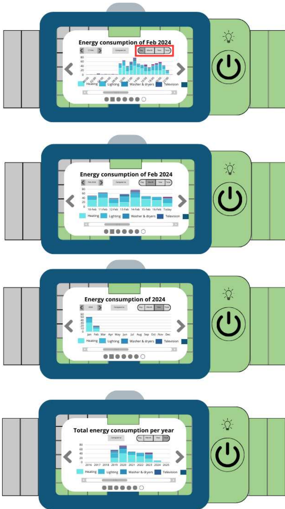
Figure 68: Illustration of the second page of the history section on the smartwatch. In the first element of the image a red box highlights the bar in which the user can tab "Day", "Month", "Year" and "Total" to go to the other elements of the figure.
