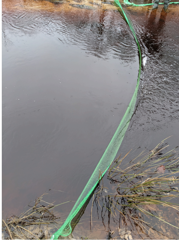
Figure 5: Photograph of the net that was spanned across the Glanerbeek to create natural surface tracers (taken by Mulder, I. on 2-2-2024)
