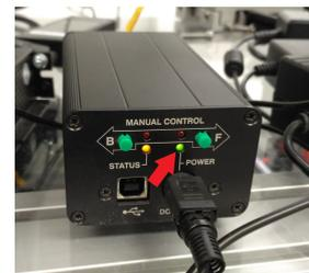
Figure A.2: Press the green buttons to rotate the halfwave plate.
