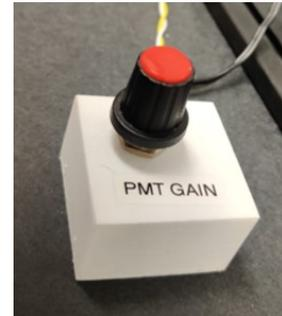
Figure A.1: Knob to change the gain of the PMT
