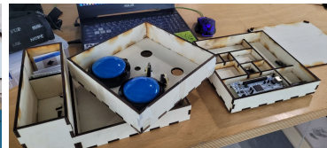
(f) The completed box with test components.
