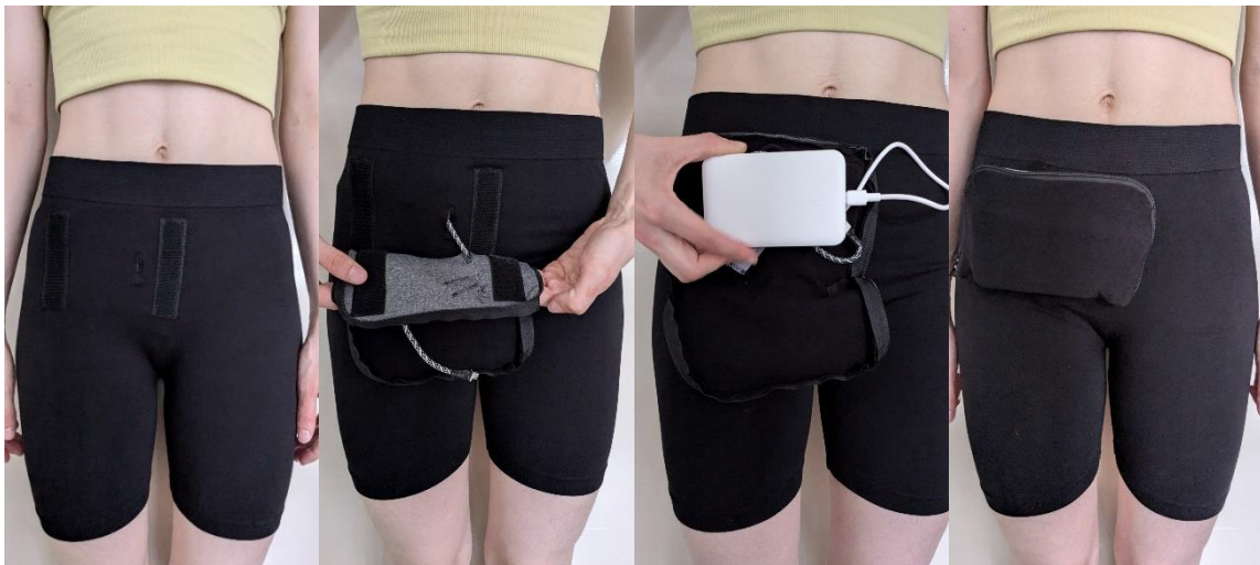
Fig. 6.19. CoreMnemo shorts worn on the body (left) and CoreMnemo shorts with the electronics pouch attached (right).
