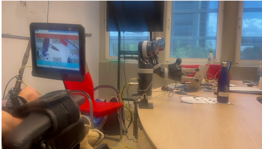
Figure 20. The client using the system via their gaze-controlled computer, attempting to pick up a bottle.
