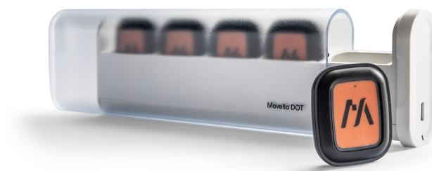
Figure 2: The Movella Dot package that uses IMUs to provide real-time data[27].
