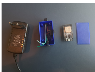
(a) The exploded view from the complete building block controlling an LED strip
