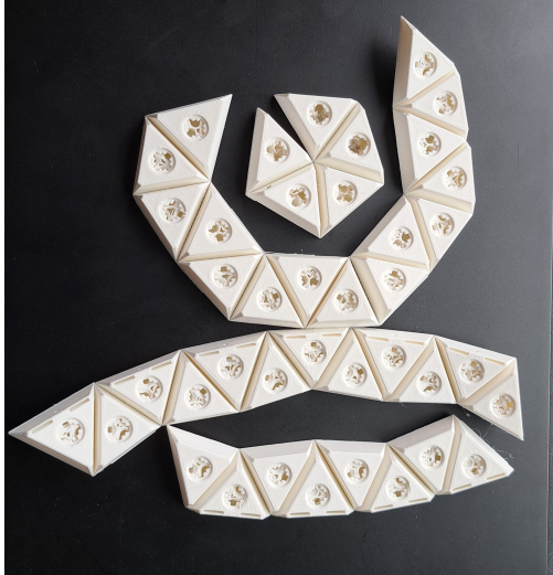
Figure 5.18: The printed LED ball components with infill. The top part consists of 5 triangles, followed by Ring 2, which contains 15 triangles surrounding the top part. The two components underneath make up Ring 3. Together, these parts represent half of the ball.
