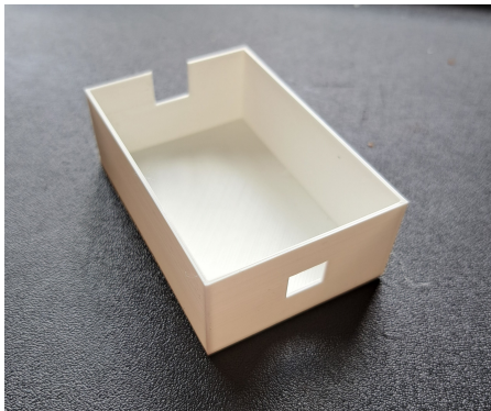
Figure 5.9: Printed version of encasing design 1 of IR tracking device
