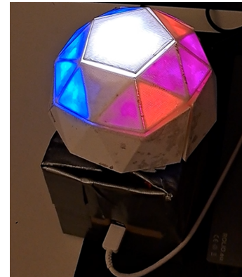
Figure 5.23: The fully assembled Ambient Sound Visualizer from the first round of iterations, featuring the half sphere and the enclosed electronics box. The red/pink side reacts to sound.
