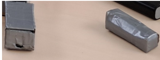
Figure 5.7: Cardboard and duct tape version of the IR transmitter and receiver. The transmitter is on the right and the receiver is on the left.
