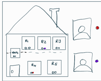
Figure 5.24: First concept drawing of the user interface of the Family Locator, designed in the shape of a house with different floors. The letter "R" represents a room number, and the two dots inside each room are individually addressable LEDs.
