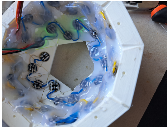
Figure 6.11: LED ball assembly process: soldering LEDs and securing with hot glue
