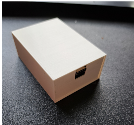
Figure 5.13: Printed version of encasing design 2 of IR tracking device
