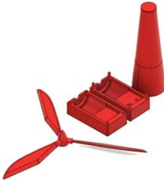
Figure 22: The 3d model used to 3d print the wind turbine
