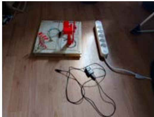
Figure 34: The setup for testing how long it takes to plug the device in
