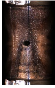
Fig. 27: Unwrapped and concatenated front- and back image.
