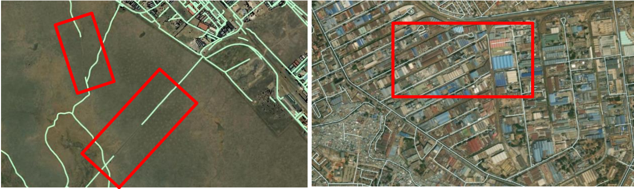
Figure 12: Images showing some instances where street segments do not connect. The street data is sourced from Microsoft Streets and Base map from Earth Geographics.
