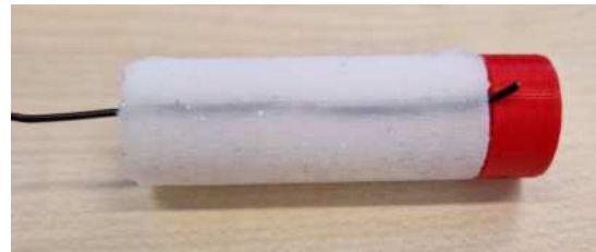
Fig. 13: Phantom finger used to test the system
