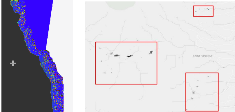
Figure 21. Noises in elevation model: on the coasts (left) and ‘fake depression’ inland (right).
