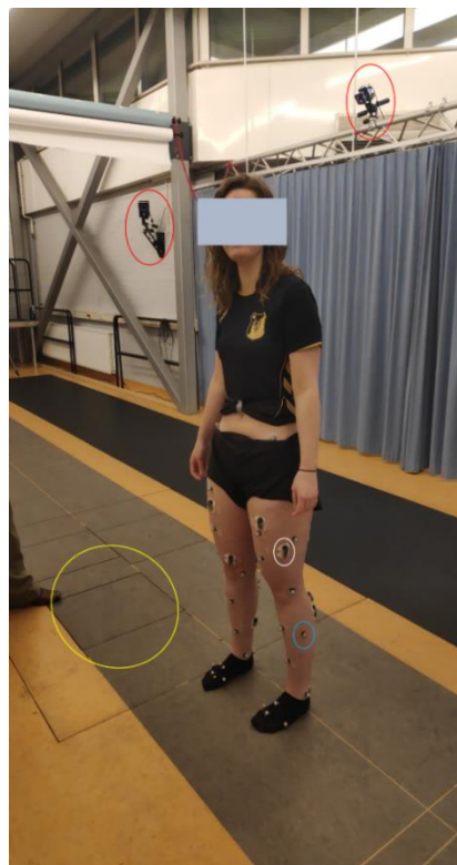
Figure 7 The pilot subject in the motion capture lab (Vicon system) in RRD center. Red circle: infrared high-speed camera, yellow circle: Force plate, white circle: EMG electrodes, blue circle: retroreflective marker.
