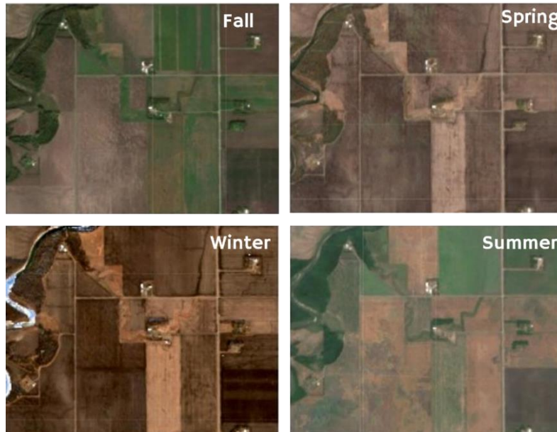
Figure 8: Qualitative example of the four seasonal Sentinel-2 composites for a specific silo's location.
