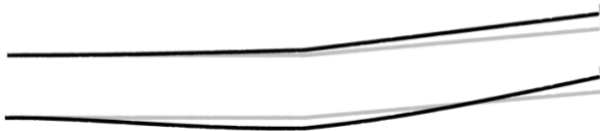
Fig. 5. Resonance modes of the probe needle. (Top) First-order resonance mode with a frequency of 108.34 Hz. (Bottom) Second-order resonance mode of the probe needle with a frequency of 684.54 Hz.
