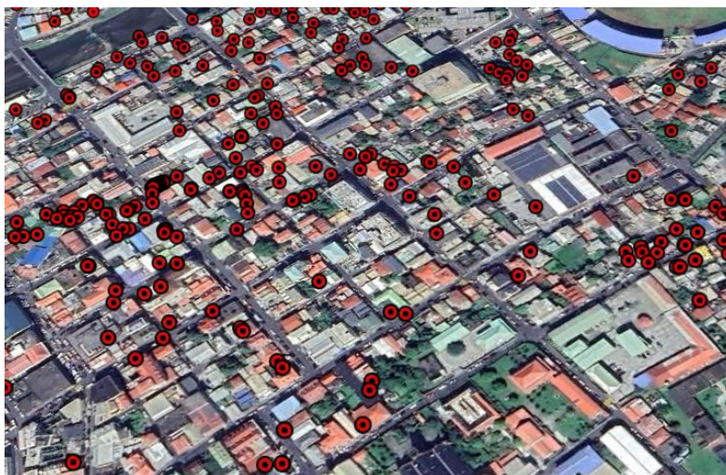
Figure 7: Overlay of GPS points for more than 75% damage for roofs in Roseau
