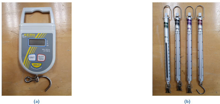
Figure 12: (a) digital Newton meter and (b) manual Newton meters of 100, 300, 600 and 2500 gram.
