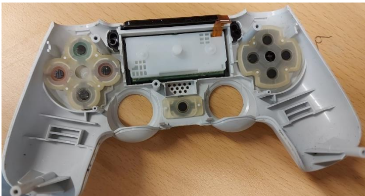
Figure 15 - Removed parts from the controller, Except the home button contact point
